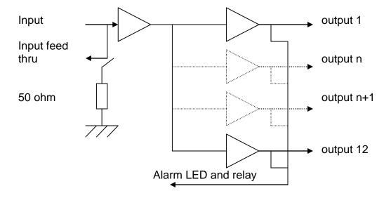
Figure 1. ptf 1204A Schematic
